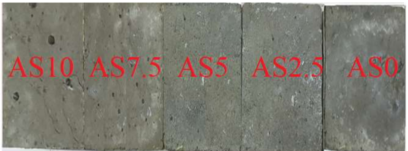
Figure 4. Visual inspection after the seawater effect
